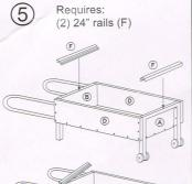
STEP 5: Take short rails (F) and snap onto end panels A&B as indicated below.
