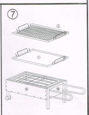
STEP 7: Lid (I) will lay on rails (E) & (F) when assembly is complete. Charcoal screen (J) will then lay on lid.
