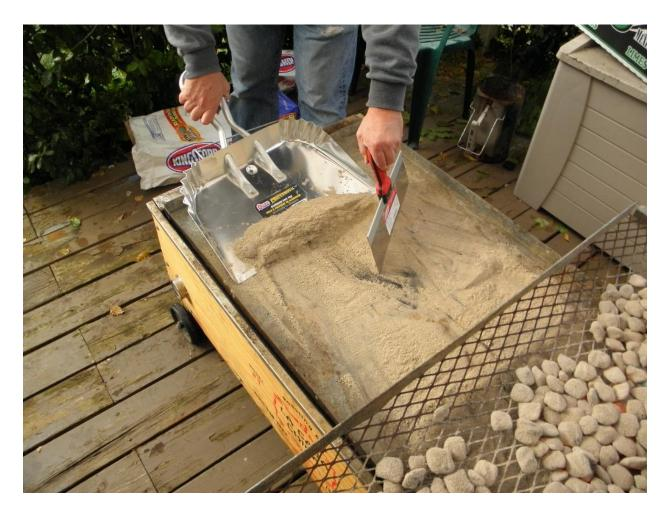
To dump ashes: Lift the charcoal grid shake it well to remove the ashes, now place it on top of two metal sawhorses. Do not place on the grass or asphalt! DO NOT Remove the ash pan from the box ~ Use a large metal scoop to pick up and dispose of the ashes.
